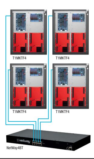
Power up to a 16 Door Access Control System with Tango PoE Driven Power supply/chargers in Trove wall mount units. Utilize stackable PDS8 power distribution boards on the Tango1B and ACM4 access power controllers for locking devices — saving valuable space. All powered by a 4-port NetWay4BT 802.3bt injector.
